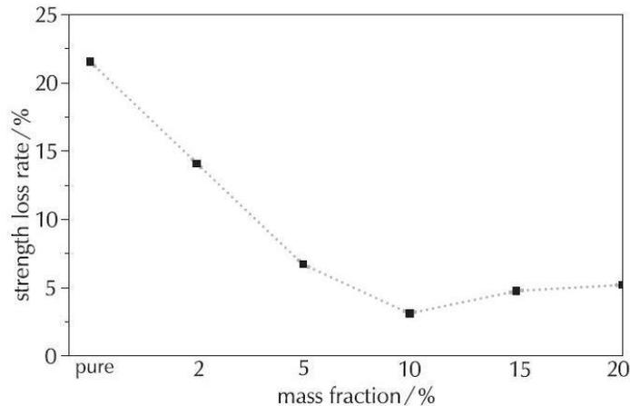
**Figure 2.** Strength loss percentage of NBR and GE-NBR after age testing. Pure NBR experiences the most strength loss, while GE-NBR experiences less % loss with varying mass fractions of graphite (Source: Li, Fei-Zhou, et al).
