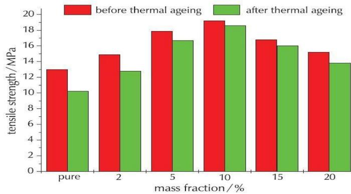
**Figure 1.** Tensile strength of NBR and GE-NBR pre and post age testing. The tensile strength of both materials decrease (Source: Li, Fei-Zhou, et al).
