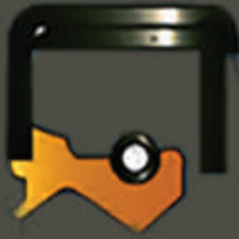
CS Outer metal case with reinforcing cap, sealing lip with garter spring and additional dust lip
