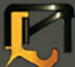
KB Outer metal case, sealing lip with additional dust lip
