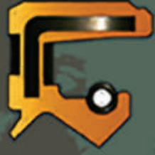
AS Rubber covered O.D., metal insert, sealing lip with garter spring and additional dust lip
