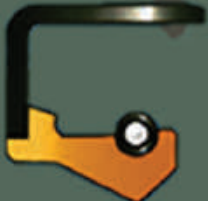
B Outer metal case, sealing lip with garter spring
