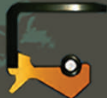
BS Outer metal case, sealing lip with garter spring and additional dust lip
