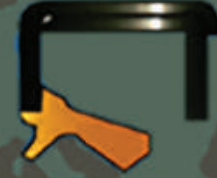
KA Outer metal case with reinforcing cap, sealing lip with additional dust lip
