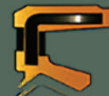
KC Rubber covered O.D., metal insert, sealing lip with additional dust lip
