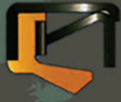
VA Outer metal case with reinforcing cap, sealing lip
