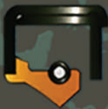
C Outer metal case with reinforcing cap, sealing lip with garter spring
