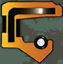
A Rubber covered O.D., metal insert, sealing lip with garter spring
