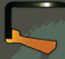
VB Outer metal case, sealing lip
