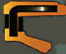
VC Rubber covered O.D., metal insert, sealing lip
