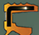
KC Rubber covered O.D., metal insert, sealing lip with additional dust lip
