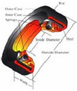
*It is almost impossible, in practice, to manufacture seal components with absolute dimensional accuracy; actual production parts may vary slightly from dimensional drawings. Given this fact, it becomes necessary that the nominal dimensions of critical contact points fall within certain acceptable ranges to allow for reliable operation.*
