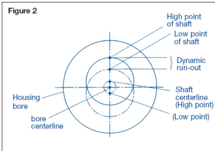
The amount of eccentricity(DRO and/or STBM) that a seal can withstand depends on the shaft speed. Typical shaft seal designs will operate satisfactorily if total eccentricity(DRO + STBM) does not exceed the maximum.
