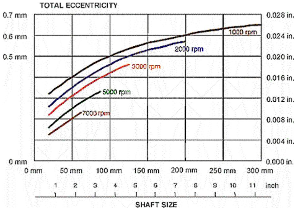
Minor variations in DRO and STBM (under 0.020 inches) have little effect upon seal torque, power consumption, pumping ability or underlip temperature. If total eccentricity is expected to exceed these limits, then special seal designs would need to be considered.
