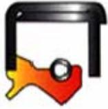
Metal OD with metal inner casing for lip protection and structural rigidity
